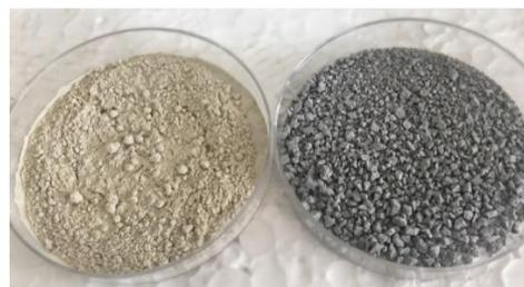
**Figure 1.** The applied soil: clay (Left) and organoclay (Right)
