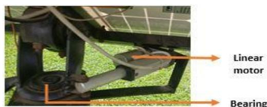
Figure 2. Linear motor for horizontal axis movement
