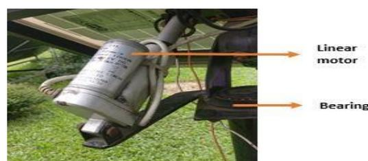
Figure 3. Linear motor for vertical axis movement
