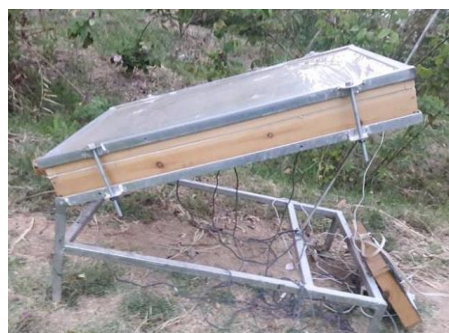
Figure. 1. Solar collector realizes for the experimental study
