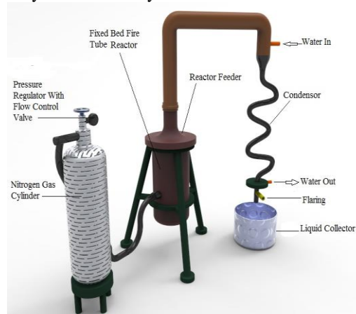
Figure 1. Schematic view of Experimental Set-up
