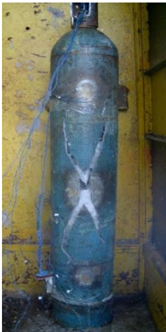
Figure 5. The crack branching in steel pressure vessel
