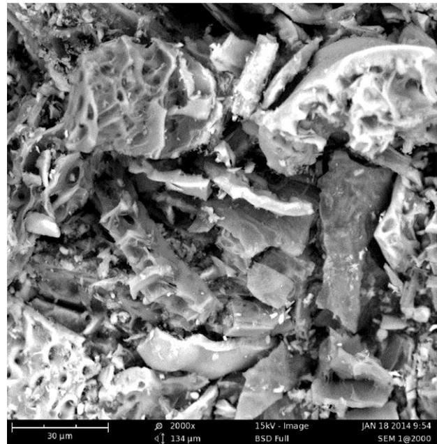
Figure 6. SEM Micrograph after acid modification
