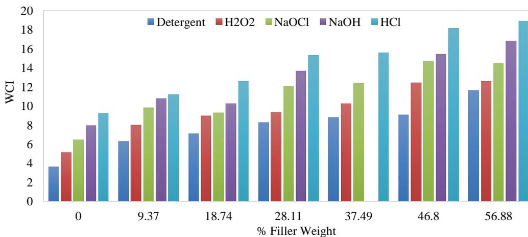
Figure 5. The Chemical Resistance of SCB-PES Composites and Control after Chemical Treatment (WCI - Weight Loss of Composites after Chemical Interaction)
