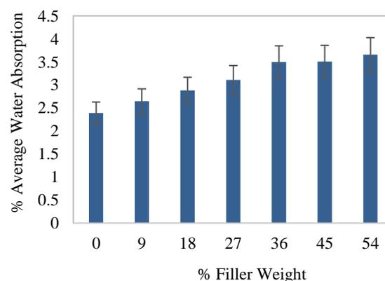
**Figure 3.** Water Absorption Rate of the Specimens after 7 Days
