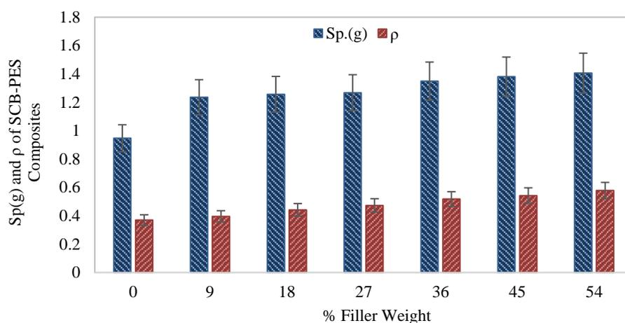
**Figure 2.** Specific Gravity (sp) / Density ( $\rho$ ) of the Specimens and Control, against % Filler Weight
