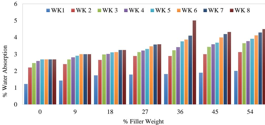
Figure 4. Merged Water Absorption Rate of SCB-PES Specimens at the end of 56 Days
