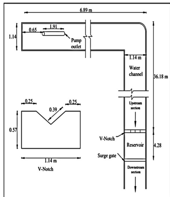
Figure 1. Plan view of the experimental setup in the lab
