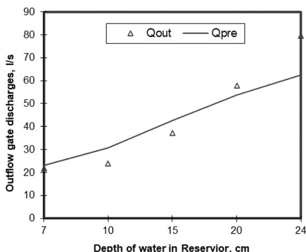
**Figure 4.** Outflow gate discharge averaged over all operating conditions
