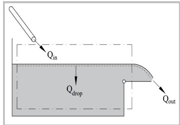
Figure 3. Control volume used in the continuity equation of the gate
