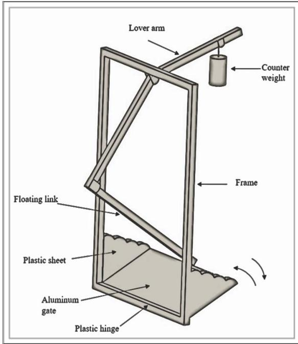
Figure 2. A schematic diagram of surge gate
