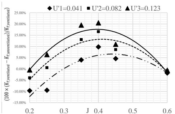
**Figure 8.** Thrust Coefficient Improvement versus Advance Coefficient for different injected Air Velocity ratio
