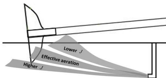
**Figure 10.** Schematic representation of effective aeration
