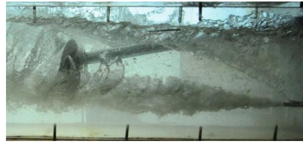
Figure 11. Effective Aeration test at U' = 0.123; \beta = 70 mm
