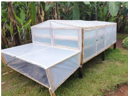
Figure 1. Direct mode dryer with wooden shelves and polythene cover
