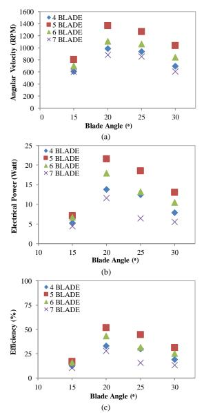
**Figure 3.** Relation between blade angle with (a) angular velocity, (b) electrical power, and (c) efficiency
