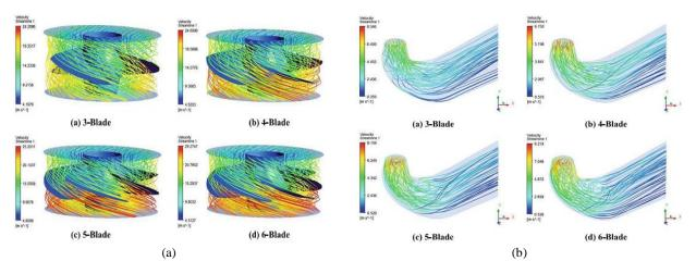
Figure 4. Sreamline in runner different solidity simulation at (a) runner (b) draftube [21]
