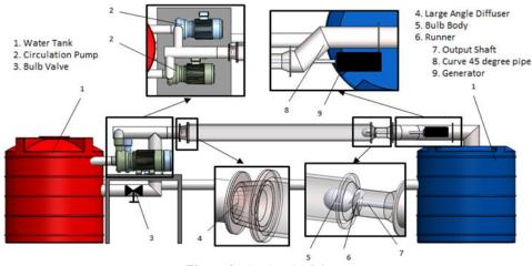
Figure 2. The sketch of rig test
