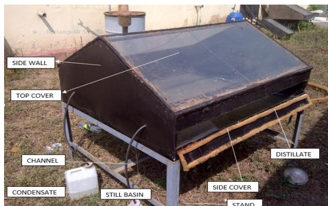
Figure 1. Experimental setup of a double slope solar still with all the components label
