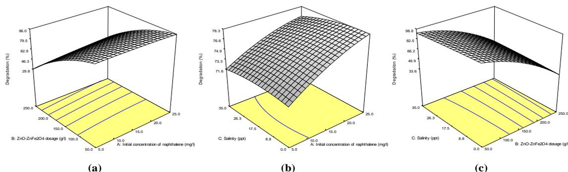
**Figure 2.** Response surface for simultaneous influence of (a) initial concentration of naphthalene and ZnO-ZnFe<sub>2</sub>O<sub>4</sub> dosage, (b) initial concentration of naphthalene and salinity, (c) ZnO-ZnFe<sub>2</sub>O<sub>4</sub> dosage and salinity
