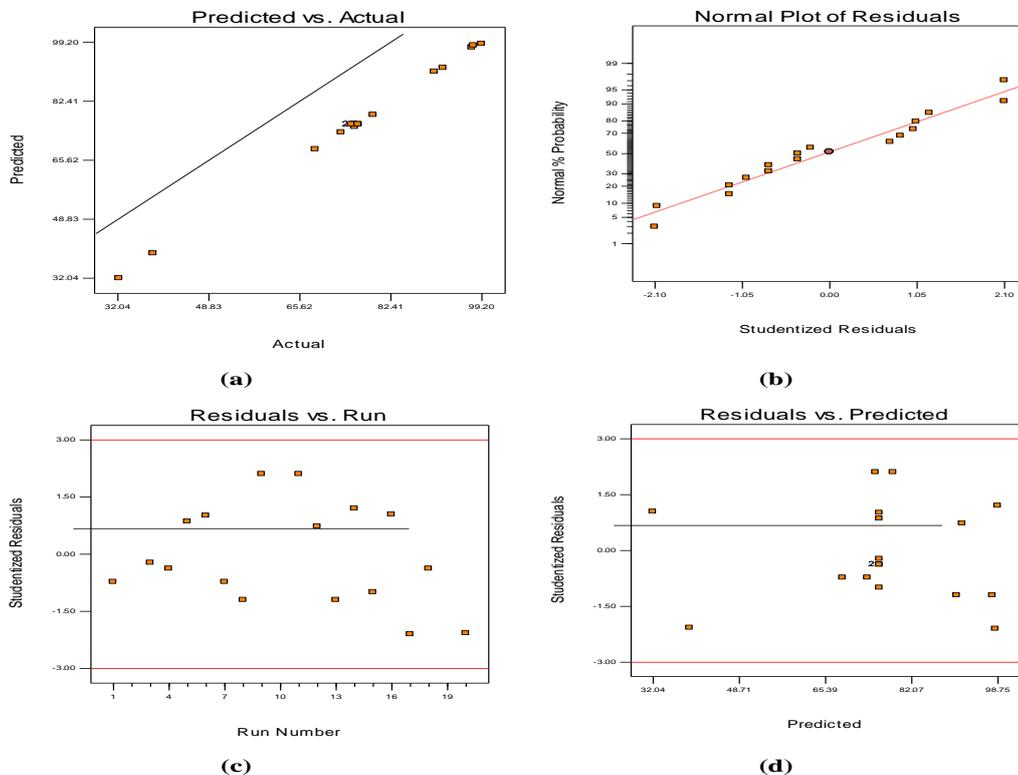
**Figure 1.** Diagnostic plots for photocatalytic degradation of naphthalene using ZnO-ZnFe<sub>2</sub>O<sub>4</sub> composite: (a) Plot of predicted against actual values, (b) Normal plot of residuals, (c) Residual versus run plot, and (d) Residual versus predicted plot
