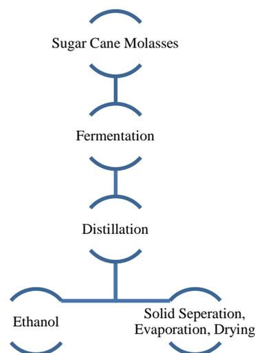
**Figure 1.** Ethanol production stages from Sugarcane Molasses
