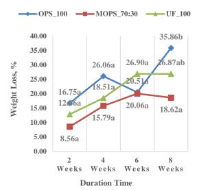
**Figure 1.** Soil burial trend analysis for particleboards bonded with native Oil palm starch (OPS\_100); modified Oil palm starch (MOPS\_70:30) and Urea formaldehyde (UF\_100). Data is expressed as means; values in parentheses show standard deviations. Values with the same letter are not significantly different (p < 0.05).
