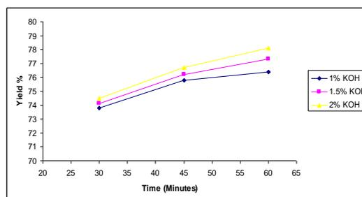
**Figure 6.** Effect of molar ratio 6:1 for biodiesel from mixture of 25% karanja and 75% linseed oil
