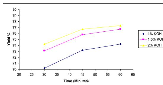
Figure 1. Effect of molar ratio 4.5:1 for biodiesel from mixture of 50% karanja and 50% linseed oil
