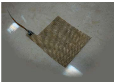
(a) Current collector
