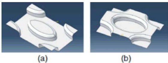
Fig. 7: Schematic of a) convex and b) concave die in ABAQUS software.
