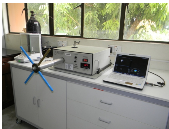
Fig. 2: Supercritical fluid technology phase behaviour monitoring system
