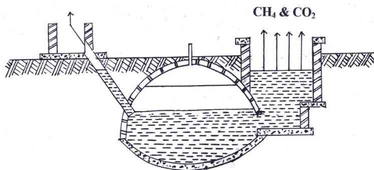
Fig. 1: CH<sub>4</sub> and CO<sub>2</sub> emission from conventional biogas plant
