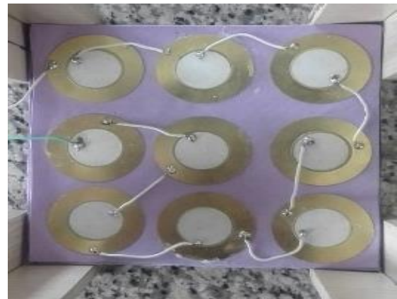
Figure 5. Schematic of piezoelectric in series connection
