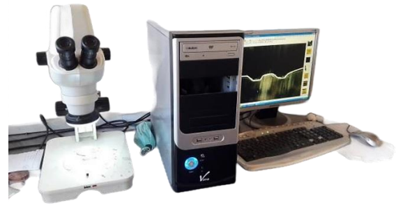
Figure 5. The used microscope to observe the formed plates and measure their thickness reduction
