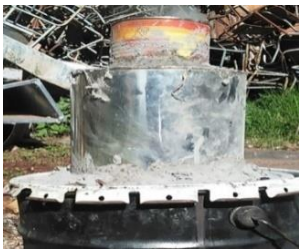
Figure 4. Carbonizer for carbonization of sample
