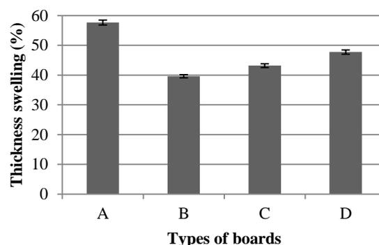
**Figure 1:** Thickness swelling of oil palm trunk particleboards.
