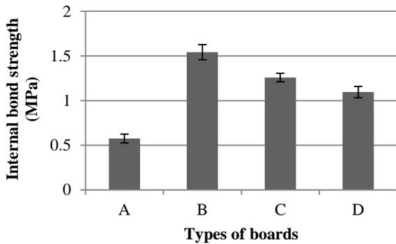
**Figure 3:** Internal bond strength of oil palm trunk particleboards.
