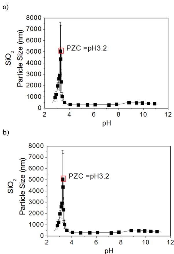
**Figure 1(a)** Surface charge of SiO<sub>2</sub> in DI water as a function of pH at a range of pH 2.5 to 11. The initial pH was found at 5.4 with a surface charge of -33 ± 2 mv. The pH of point of zero charge (PZC) was identified at 3.2. **(b)** Particle size measurement of SiO<sub>2</sub> in DI water as a function of pH at a range of pH 2.5 to 11. The initial pH was found at 5.4 with a particle size of 296 ± 19 nm. The pH of point of zero charge (PZC) was identified at 3.2.
