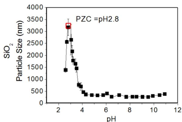
**Figure 3(a)** Surface charge of SiO<sub>2</sub> in tap water as a function of pH at a range of pH 2.5 to 11. The initial pH was found at 7.1 with a zeta potential of  $-27 \pm 2$  mv. The pH of point of zero charge (PZC) was identified at 2.8. **(b)** Particle size
