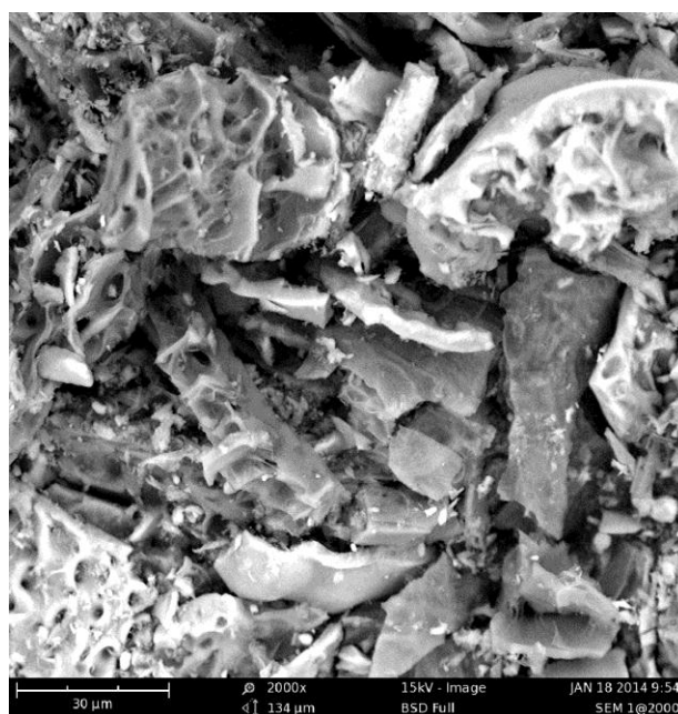
Figure 6. SEM Micrograph after acid modification
