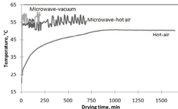
Fig. 4: Product temperature progressions during drying process
