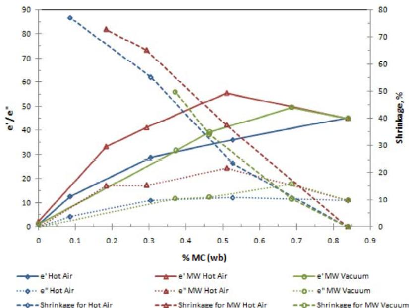
Fig. 7: Influence of dielectric constant ( $\epsilon'$ ), dielectric loss factor ( $\epsilon''$ ) and volume shrinkage on the moisture content of red pitaya slices dried in three different drying systems: hot air dryer, microwave-hot air dryer and microwave-vacuum dryer
