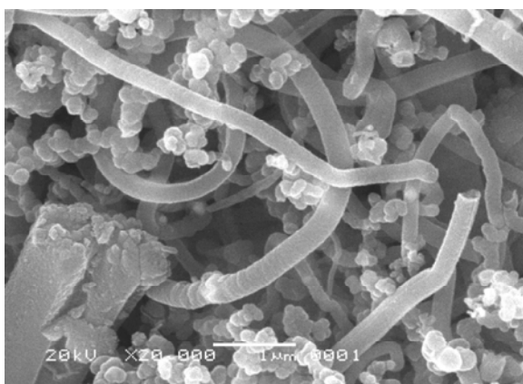
Fig. 2: Cross-sectional FESEM images of modified multi walled carbon nanotubes (MWNTs)
