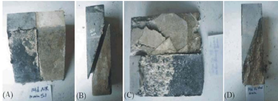
A= Interface failure, B = Interface failure & substrate cracks, C = Interface failure & substrate fracture, D = Substratum failure.
