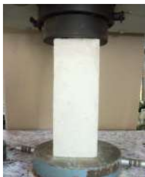
Fig. 1: Specimen for OC compression test
