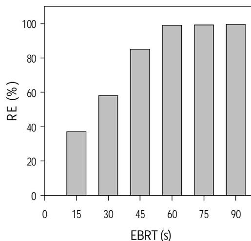
Fig. 3: Removal efficiency of ethyl acetate at different EBRTs (inlet concentration of 150 ppm)
