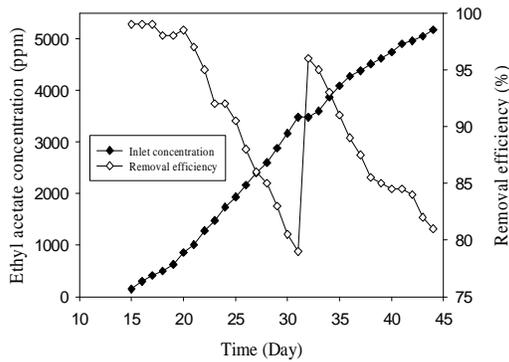
Fig. 4: Biofilter performance for ethyl acetate removal
