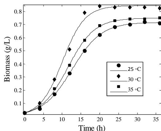
Fig. 2: Cell dry weight of *P. putida* at different temperature for ethyl acetate concentration of 1 g/L
