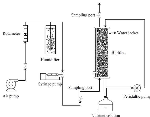
Fig. 1: Schematic diagram of the biofilter used for the removal of ethyl acetate
