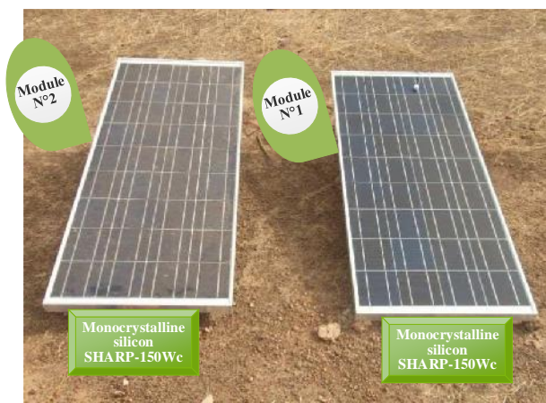
Figure 3. Study of Dust Deposit: Experimental Setup
