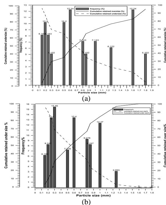
**Figure 6.** (a) Histogram, % cumulative retained oversize, under size and frequency versus grain size of the corn cob, (b) Histogram, % cumulative retained oversize, under size and frequency versus grain size of wheat dust powder
