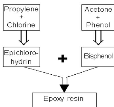
Figure 2. The composition of Epoxy
