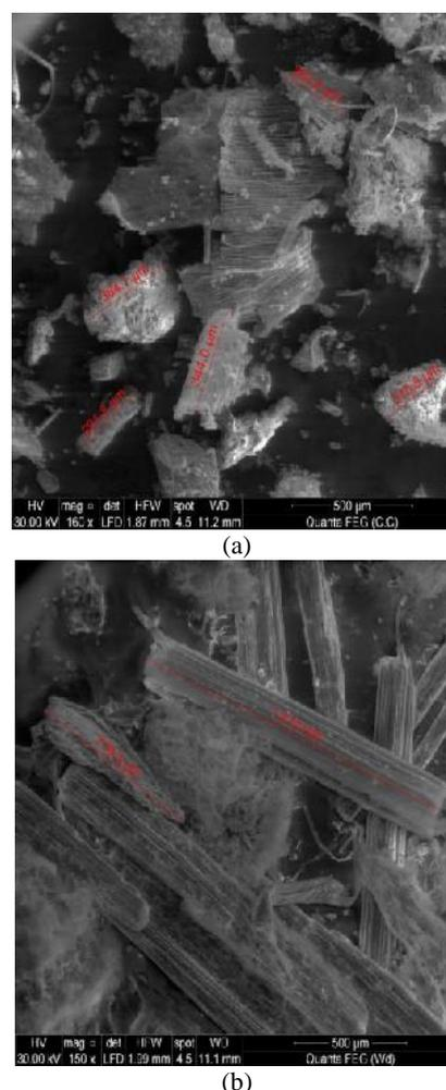
**Figure 8.** Scanned image of crushed corn cob, (b) Scanned image of wheat dust this stage. Due to the exothermic quality of this process, the additional heat permits the emission of remaining.
