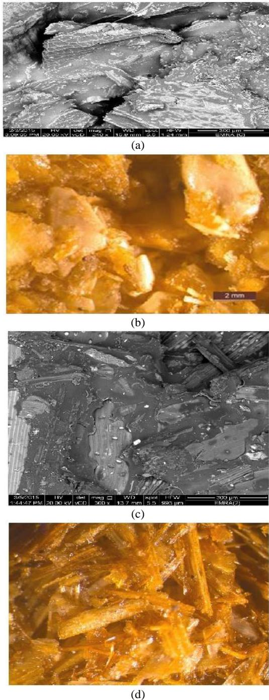
**Figure 9.** Scanning electron microscopic image of the outer surface of corn cob pellets, (b) Micrograph image of the outer surface of corn cob pellets, (c) Scanning electron image of the outer surface of wheat dust pellets, (d) Micrograph image of the outer surface of wheat dust pellets
