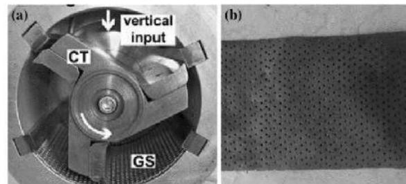
**Figure 1.** The cutting mill machine used in the second stage of milling, b the GS
