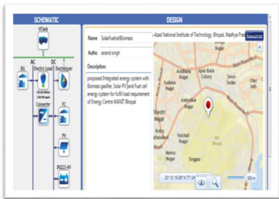
Figure 3. HOMER simulation model of solar PV, biomass gasifier generator set, and fuel cell hybrid energy system
