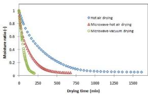
Fig. 3: Drying curves of red pitaya slices
