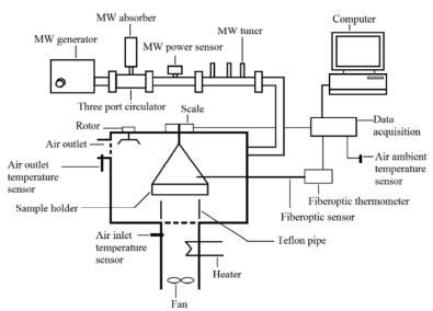
Fig. 1: Schematic diagram of microwave-hot air drying
