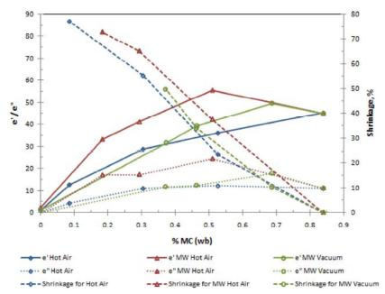
Fig. 7: Influence of dielectric constant ( $\epsilon$ '), dielectric loss factor ( $\epsilon$ '') and volume shrinkage on the moisture content of red pitaya slices dried in three different drying systems: hot air dryer, microwave-hot air dryer and microwave-vacuum dryer
