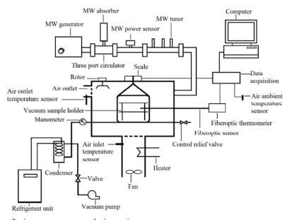
Fig. 2: Schematic diagram of microwave-vacuum drying unit
