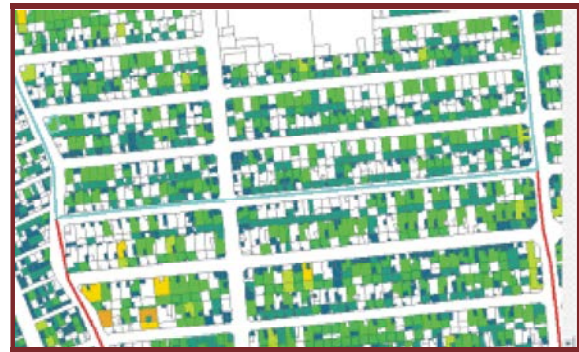
Fig. 2: A portion of the 1:2000 urban digital map comprising of parcel data
