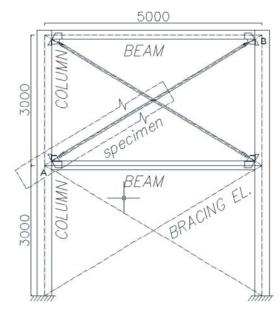
Fig. 3: Specimen cut
