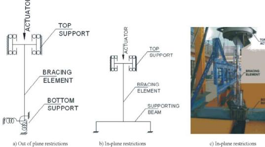
Fig. 4: Test setup and support restraints
