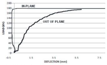
Fig. 6: Load-lateral deflection in mid height of specimen
