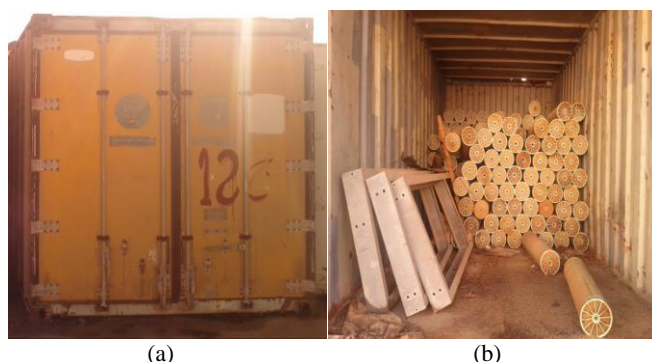
Figure 2. The container (a) and used membranes installed in a container (b)
