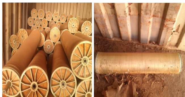
Figure 3. Used membrane cells
