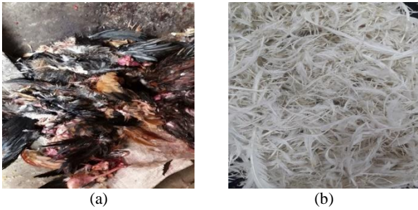
Figure 2. Waste chicken feather; a) Feather waste in slaughterhouse and b) Cleaned and dried feather waste
