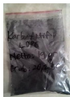
Figure 7. The results of Activated Carbon from pyrolysis oil of LDPE plastics waste
