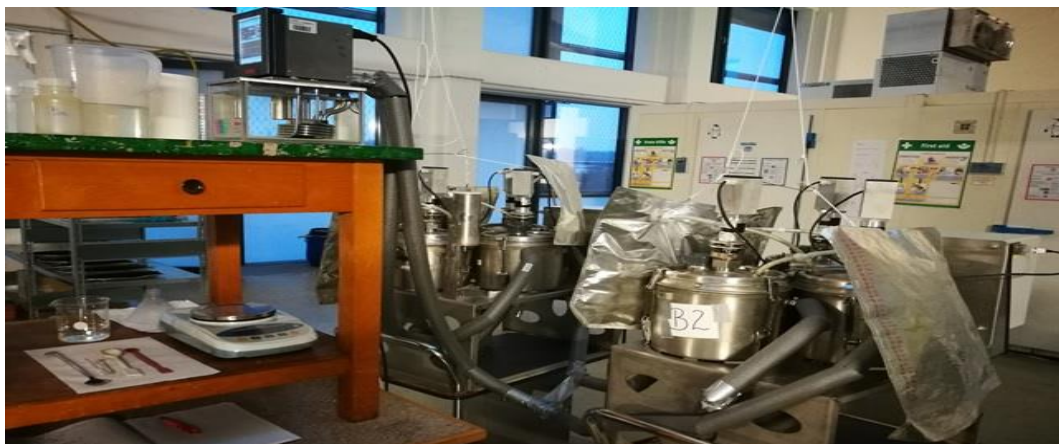
Figure 6. AD reactors in lab-scale at IAK
