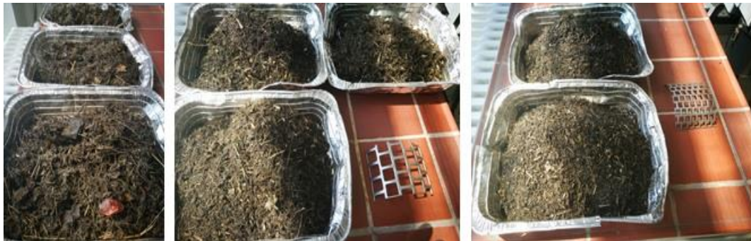
Figure 5. Dried and grinded bio-waste in different particle sizes
