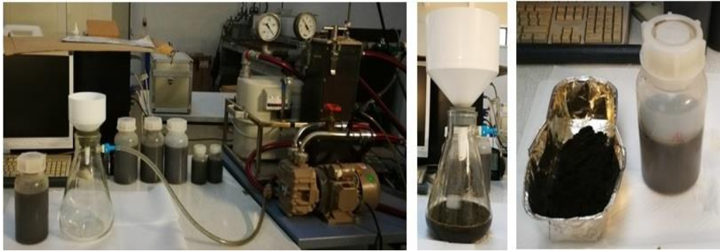
Figure 7. Dewatering of digestate
