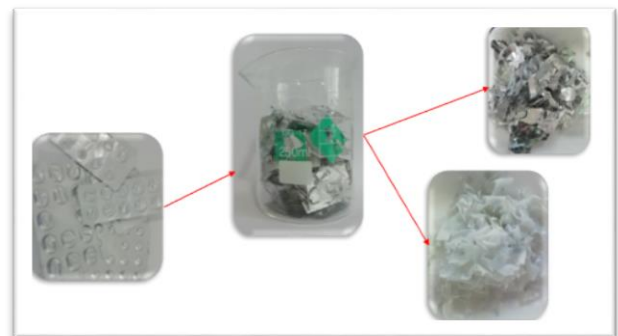
Figure 3. Separation of pharmaceutical blisters
