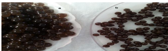
Figure 9. (a) AMCBCC treated with NaOH, (b) AMCBCC treated with HCl
