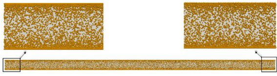
Figure 9. Particle Deposition in a Simple Microchannel with Developed Inlet Velocity
