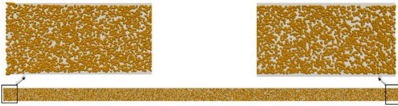
Figure 10. Particle Deposition in a Simple Microchannel with Uniform Inlet Velocity
