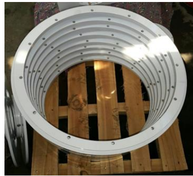
Figure 7. The stator rings after machining process
