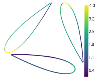
Figure 2. Y^+ on blade walls in TSR = 2.64
