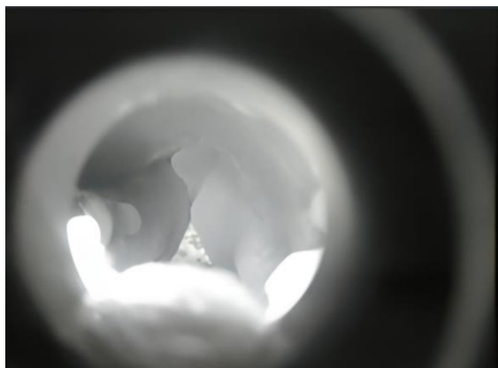
Figure 2. A real image of methane hydrate formed in a laboratory reactor
