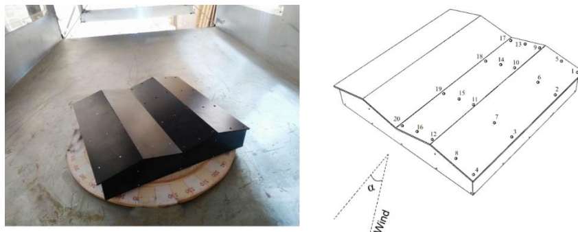
Figure 4. The pressure measurement points in the wind tunnel test on two-span shed structure
