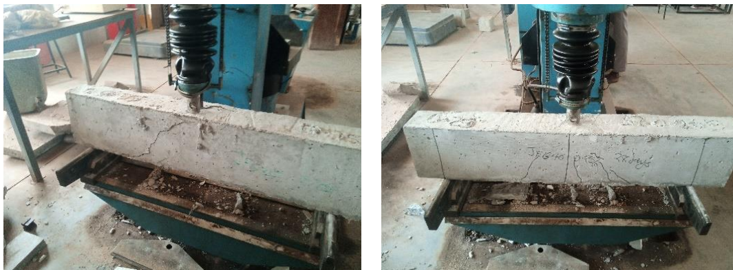
Figure 5. The diagonal crack developed during the Shear beam test
