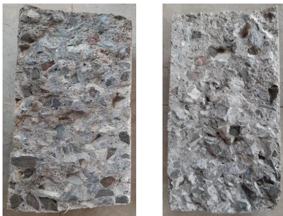
Figure 5. Tensile strength test at 365 (left) and 28 days (right)
