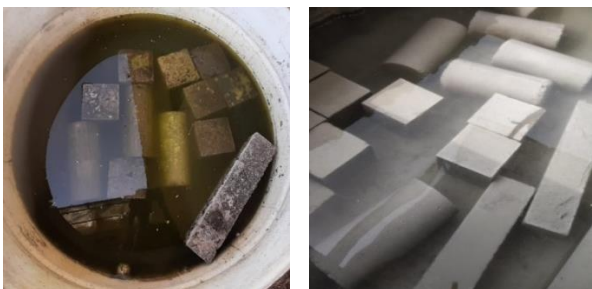
Figure 2. Curing of specimens in waste and fresh water
