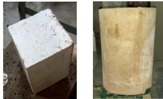
Figure 11. Color changes of samples after heating
