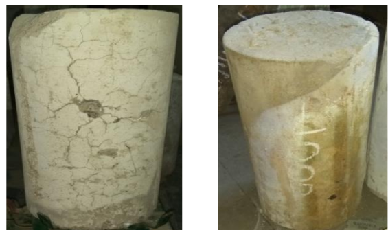
Figure 12. Thermal cracking on typical cylinder
