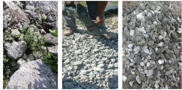
Figure 1. Recycled concrete aggregates from C & D waste
